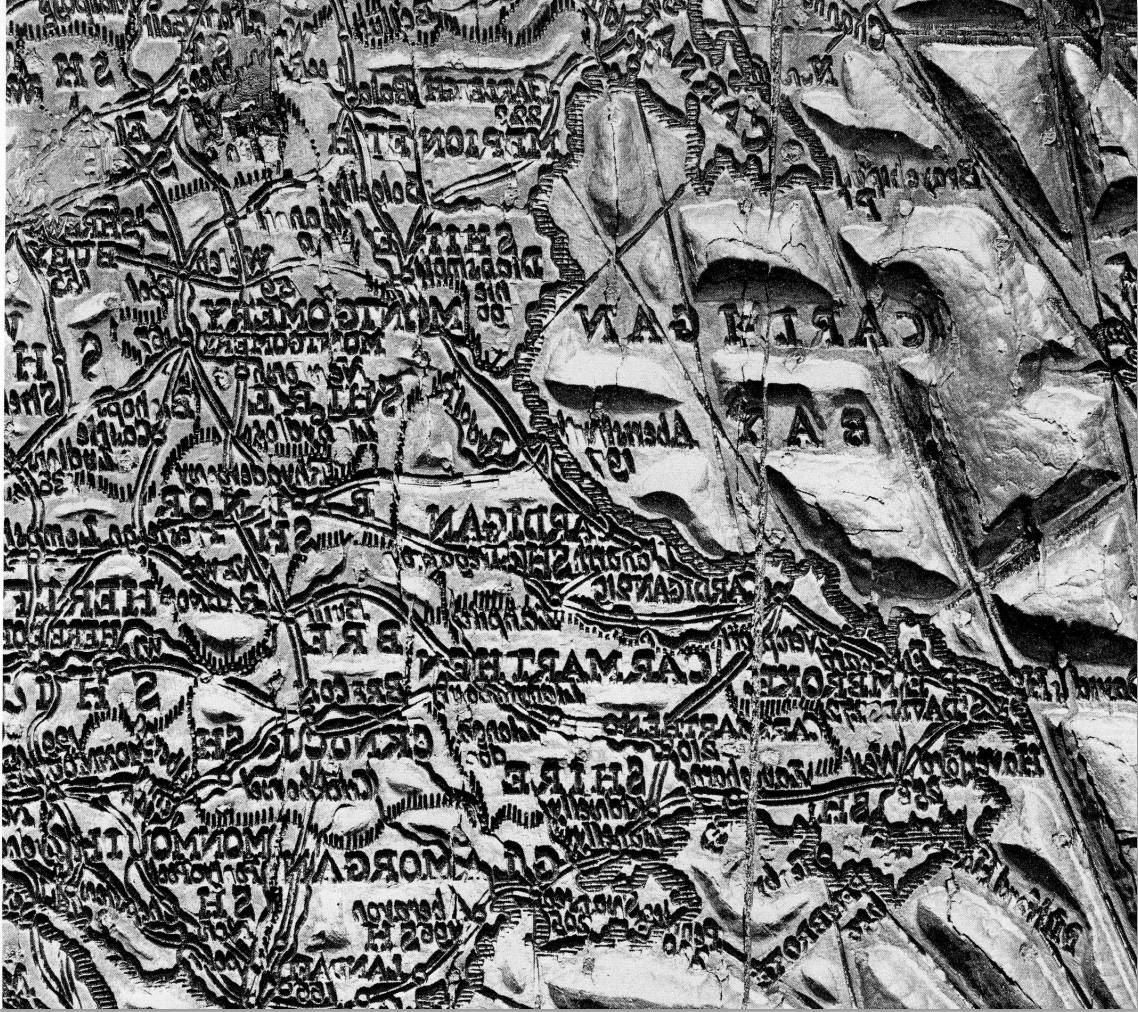
Part of the original wood block used to print A New Map of England and Wales with ye Roads & Distances of ye Principal Towns in Measur'd Miles from London [ca. 1800?]. Note that the words are engraved in a "mirror image" (i.e., backwards)
